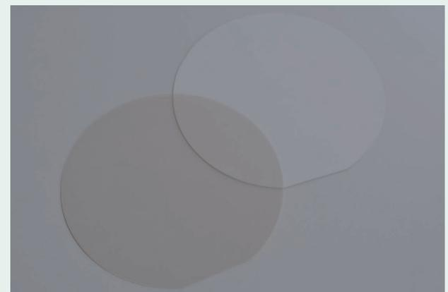
LiNbO<sub>3</sub> 4inchウエハ (研磨後、研磨前)
